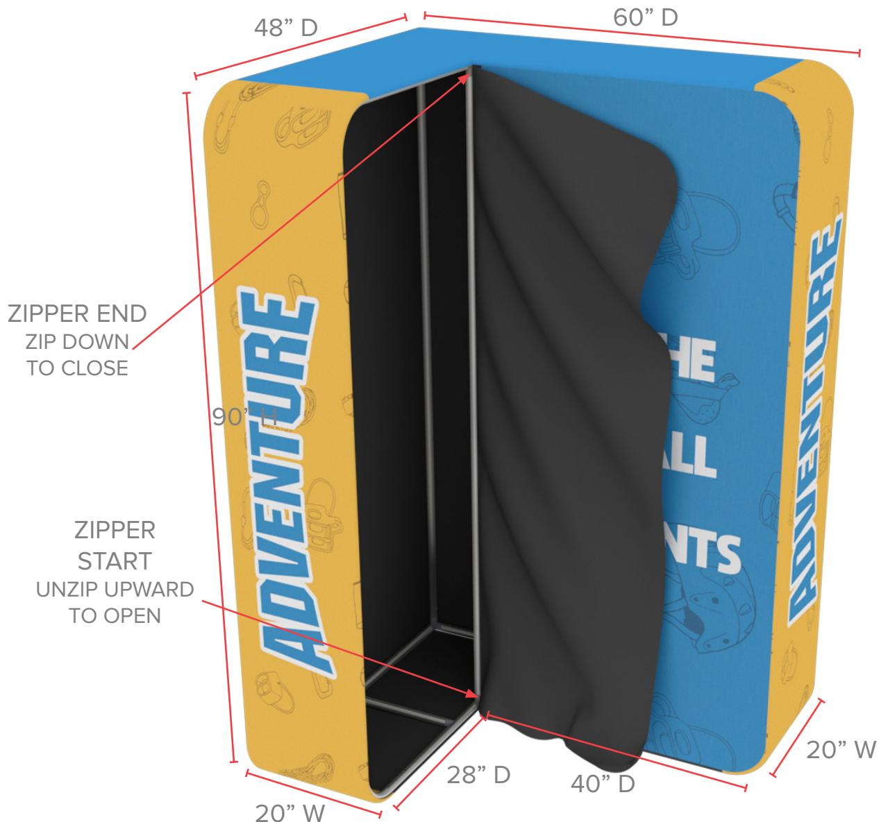
Storage area is located on the left hand side of the display and is accessed via a zipper on the front face of the graphic. The zipper opens from the bottom up, starting from the corner where the front graphic meets the storage area and runs up along the end cap seam. Zipper color is white so keep that in mind when designing graphics.
