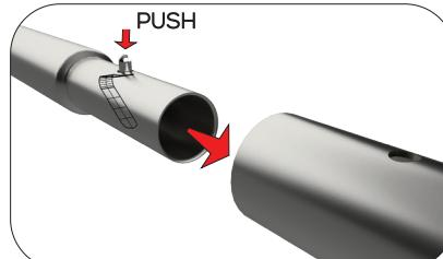
Press button & insert swaged end into receiving end of tubing
