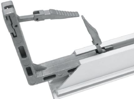
Tool free corner locks (RESORT-TFCRNR) are utilized to connect the bottom corners of the frame. Simply slide the lock into the spines of the VAIL-120DB profiles and press down levers to lock them into place.
