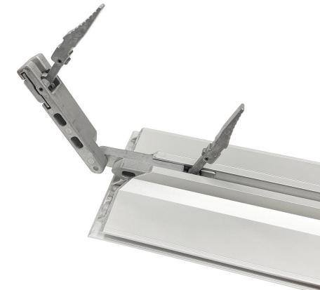
Variable angle tool free corner locks (LOCK-018) are utilized to connect the top corners of the frame at various angles outside of the standard 90° connection. Simply slide the lock into the spines of the VAIL-120DB profiles and press down levers to lock them into place.
