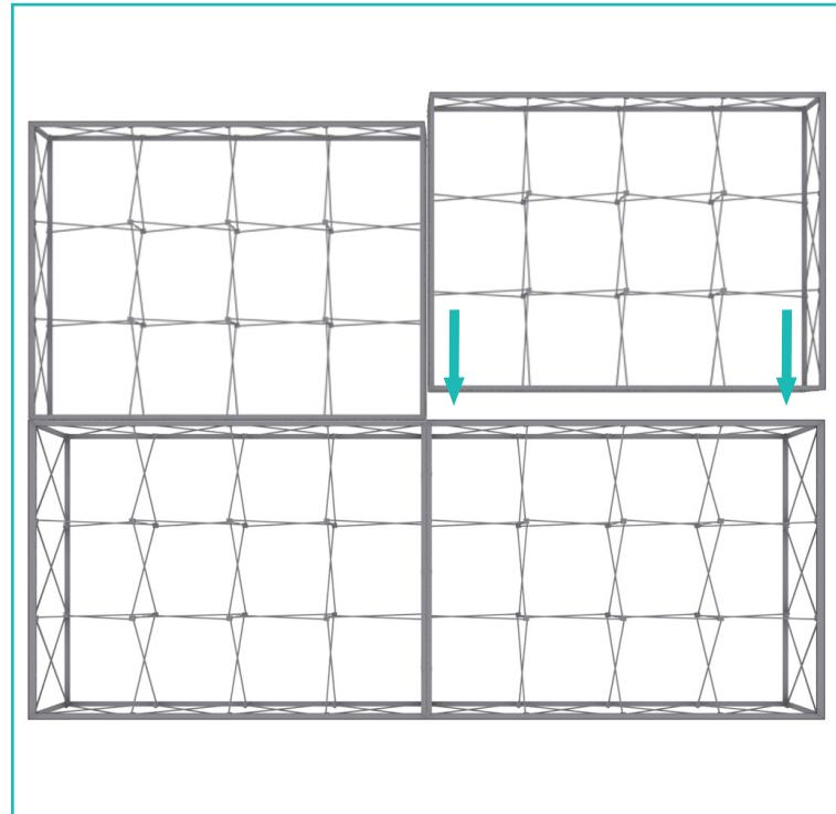
**Note:** Rendering shown without graphics for clarity. 4x3 front side graphics must be installed first before placing the frames on top.
