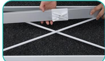
a. Clip dual edge lights to bottom X braces of frame. There should be 1 light strip per section of the frame.
