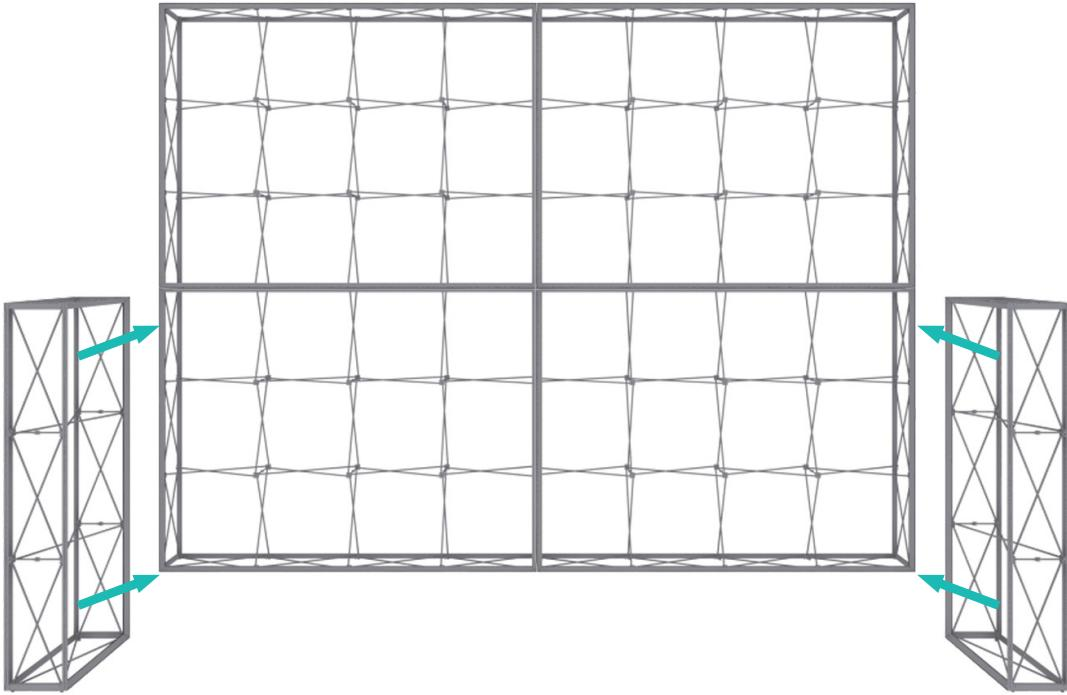
Adjoin the 1x3 frame perpendicular (90° angle) to the front side of the 4x3 frame.
