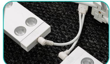
b. Plug Y cables into ports on the ends of the edge light strips. Each Y cable will connect two led strips together. Plug each Y cable into the transformers to complete dual edge light wiring.
