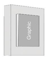
Install your graphic by tucking the silicone beading into each corner of the frame and then working your way around the edges of the frame to complete graphic installation.
