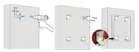
Position the wall mounts on the wall close enough for the threaded screw to be able to apply pressure to the frame. Space them evenly across the top and bottom edges of the inside edges of the frame. Mark the hole locations with a pen or marker and drill holes large enough to fit the plastic screw anchors.
